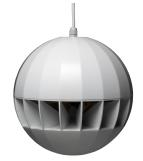
The Apart SPH20 is dual cone 100 volt sphere loudspeaker with a built-in special dispersion cone which gives you a 360° wide dispersion. These speakers allow a loud and wide sound dispersion to be produced with a minimal number of loudspeakers. SPH20 is the most cost-effective solution for background music or speech in installations with high ceilings where you need to cover an expansive area (warehouses, supermarkets, industrial buildings...).
